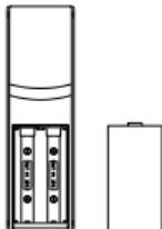
The temperature transmitter uses 2 x AA, IEC LR6, 1.5V batteries. To install and replace the batteries, please follow the steps below:
