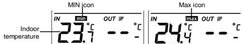
5. Press the MIN/MAX/+ to return to current indoor and outdoor temperature display.
