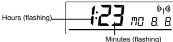
1. The hour digit in the time section starts flashing. Use the MIN/MAX/+ key to set the hour.
