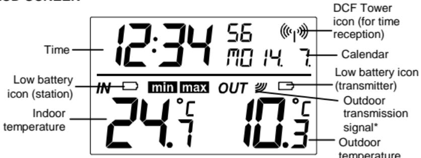
\* When the signal is successfully received by the temperature station, the outdoor transmission icon will be switched on. (If not successful, the icon will not be shown on LCD). The user can then easily see whether the last reception was successful (icon on) or not (icon off). On the other hand, the short blinking of the icon shows that a reception is currently taking place.
