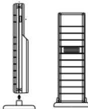
The transmitter is supplied with a holder that may be attached to a wall with the two screws supplied. The transmitter can also be positioned on a flat surface by securing the stand to the bottom to the transmitter.
