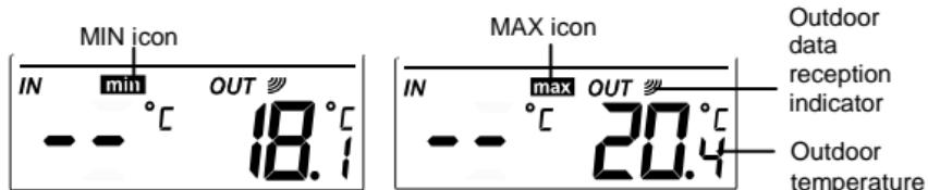
3. Press the MIN/MAX/+ key a third time to show the indoor MIN display and the time and date of record.
